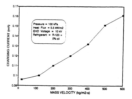
Fig. 13 Mass velocity vs. the EHD current for the in-tube boiling test section
