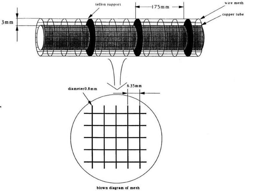
Figure 3: Details of wire mesh electrode surrounding the hot water tube
