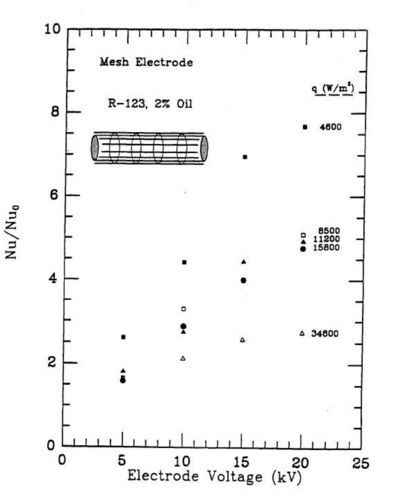
Fig. 5 EHD-enhanced external boiling of R-123 with wire mesh electrode at 2% oil
