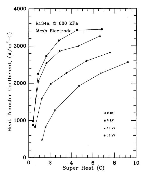
Fig. 7 EHD-enhanced external boiling of R-134a at P=680 kPa and  $T_{sat}$ .=25.85°C
