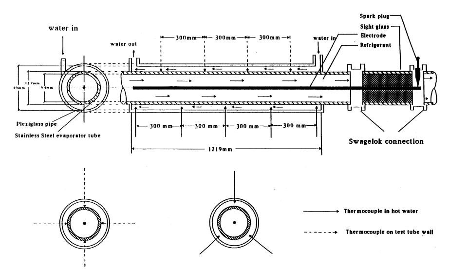
Fig. 10 Layout of lest rig showing thermocouple locations
