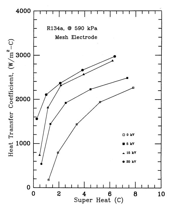
Fig. 6 EHD-enhanced external boiling of R-134a at P=590 kPa and  $T_{sat}$ =20.85°C
