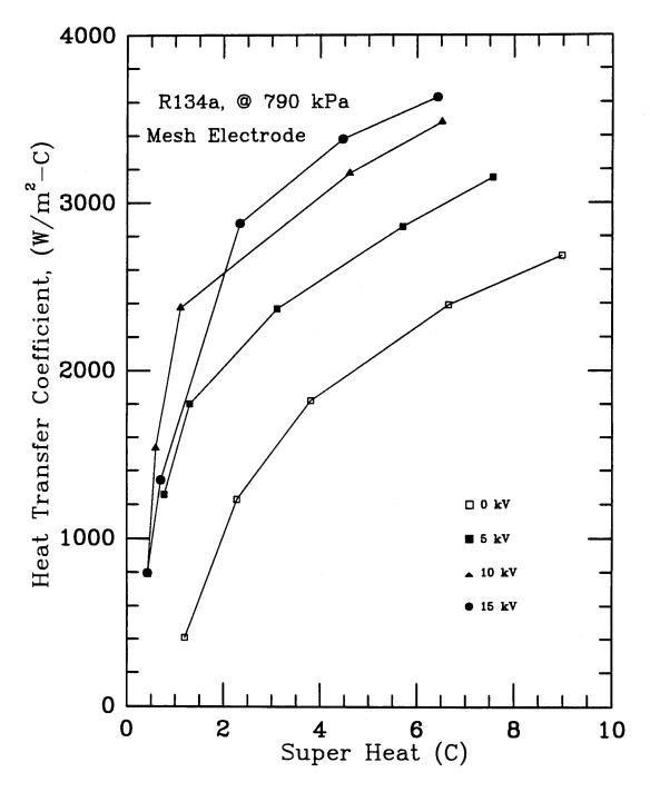
Fig. 8 EHD-enhanced external boiling of R-134a at P=790 kPa and  $T_{sat}$ =30.85°C
