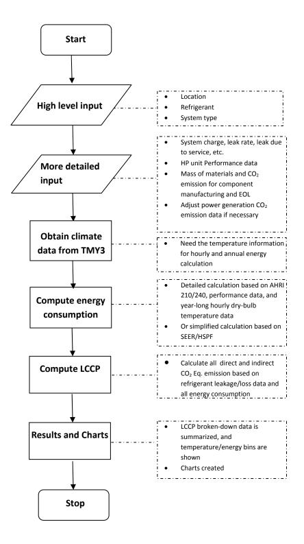
Figure 2: Flowchart for LCCP calculation
