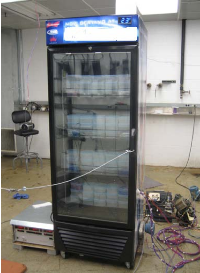
Fig 2. Model ARV-570 used for drop-in tests Note discharge air temperature display in upper right reads 23°F (-5°C)
