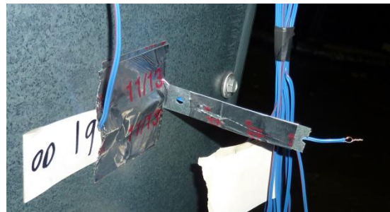
Figure C11. Typical Thermocouple Temperature Measuring Device Mounting
